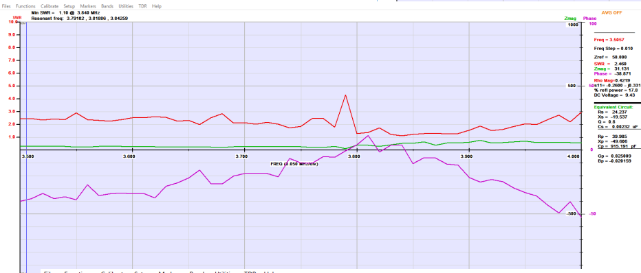
Figure 9 [left] 80m scan - note the RED line for SWR
