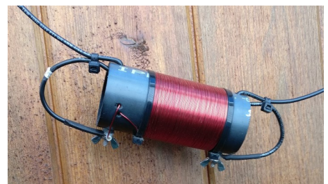
Figure 5 - Loading coil on 2" PVC
