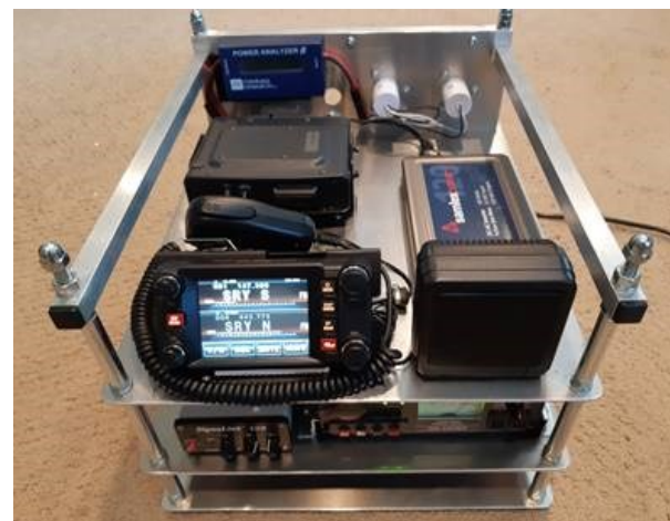
[Above] Front view of largely complete go kit. Voltage-power meter is at left rear. [Below] Go kit inside its case.
