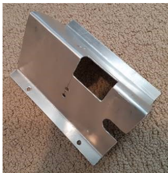
Home-made bracket for the radio control head.
