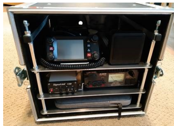
[Above] Front view of largely complete go kit. Voltage-power meter is at left rear. [Below] Go kit inside its case.
