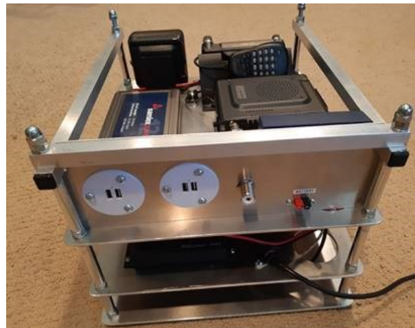
Rear view of the go-kit showing the USB charger, coax and battery ports.
