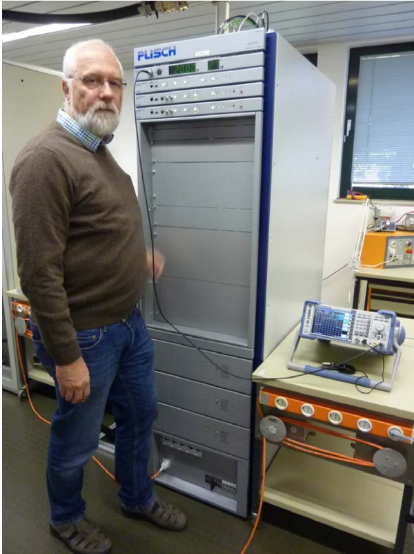
Uwe Krüger uses Rohde & Schwarz ETL signal analyzer to test the Plisch DAB+ transmitter installed at the broadcaster's Witthoh site (close to the border between Germany and Switzerland).
