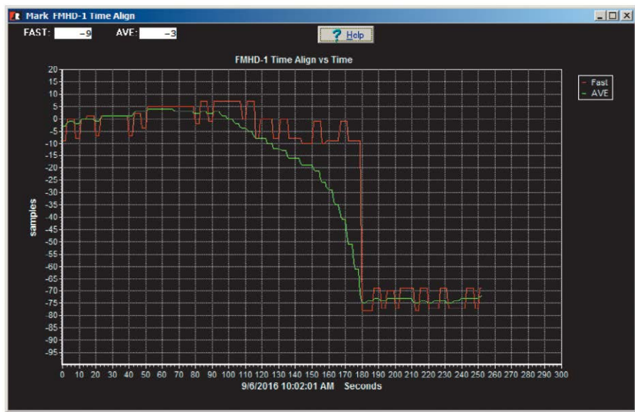
Fig. 2: Graph shows a delay correction applied to the audio processor by the Belar FMHD-1.
